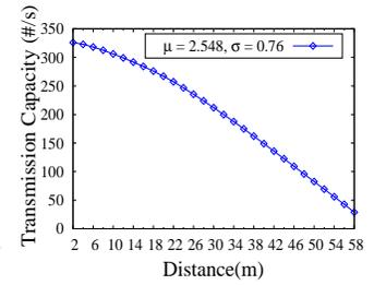
Fig. 5: Transmission Capacity with  $d_{ROI} = 50m$  and  $\xi_p = 0.99$
