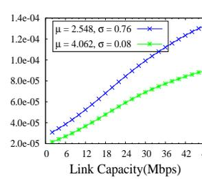
Fig. 4: PDF of Link capacity of VANET broadcast
