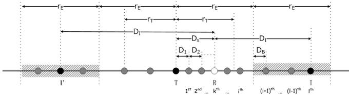
Fig. 1: General interfering scenario for VANET safety message broadcast
