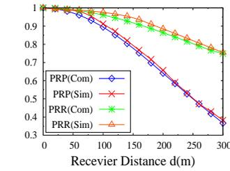
Fig. 3: PRP and PRR of VANET with NS2 simulation ( $\mu = 2.548$ ,  $\lambda = 10pkt/s$ )
