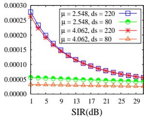
Fig. 2: Conditional PDF of SIR at receiver
